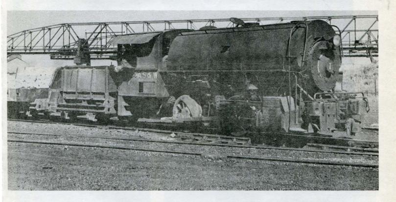
AS&W #7 about to shove a train of charging buggies containing ore and limestone up the "Highline", to the open-hearth in the early 1950's. This little saddle-tank 0-4-0 was built by Porter in 1915 for the Minnesota Steel Co. Small but mighty, she tips the scales at almost 40 tons.
