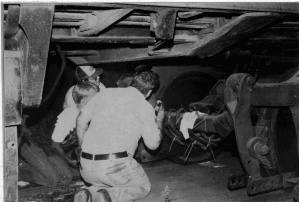
Tom Dorin, Kent Rengo and Marty Fair crawl under the 2500A to check out the condition of the traction motors and connecting electrical cables.
