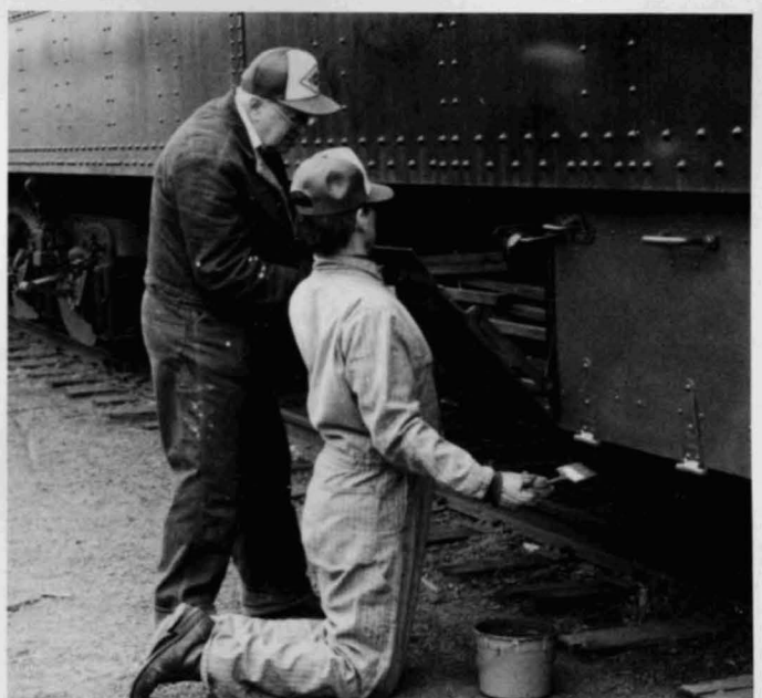
Bill Mickelsen and Bob Sailstad paint the battery box of the LS&M coach 85 in preparation for the summer's activities.
